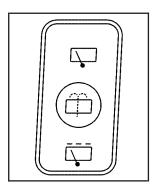
The switch for the rear washer/wiper is located in the overhead console.  $\bigtriangledown$  (**Rear Wiper**): Press this side of the button to turn the rear wiper on.
